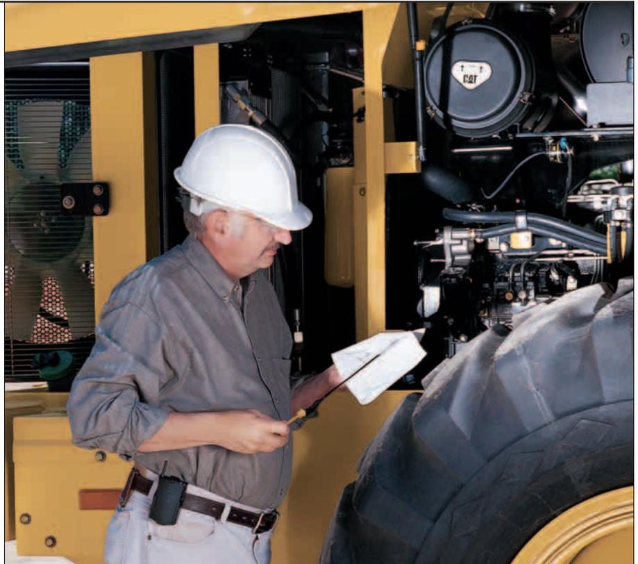
**Self-Diagnostics.** Self-diagnostic transmission and data link allows quick and easy troubleshooting by service personnel. Service codes are easily accessed through the gauge console.
