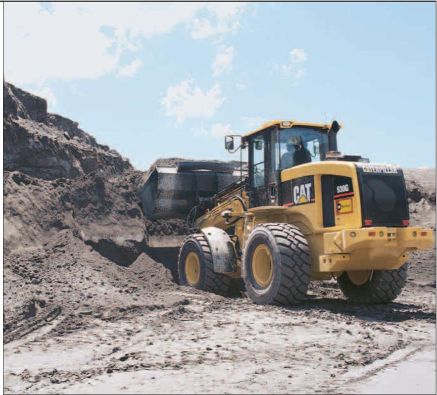
**Service Intervals.** The normal engine oil change requirement is every 500 hours of operation.
