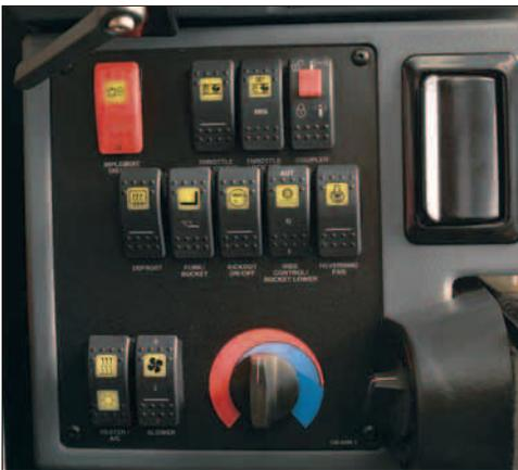
**Instrument Panel.** The 930G instrument panel is conveniently located with easy-to-read gauges and expanded warning/indicator and diagnostic functions.
