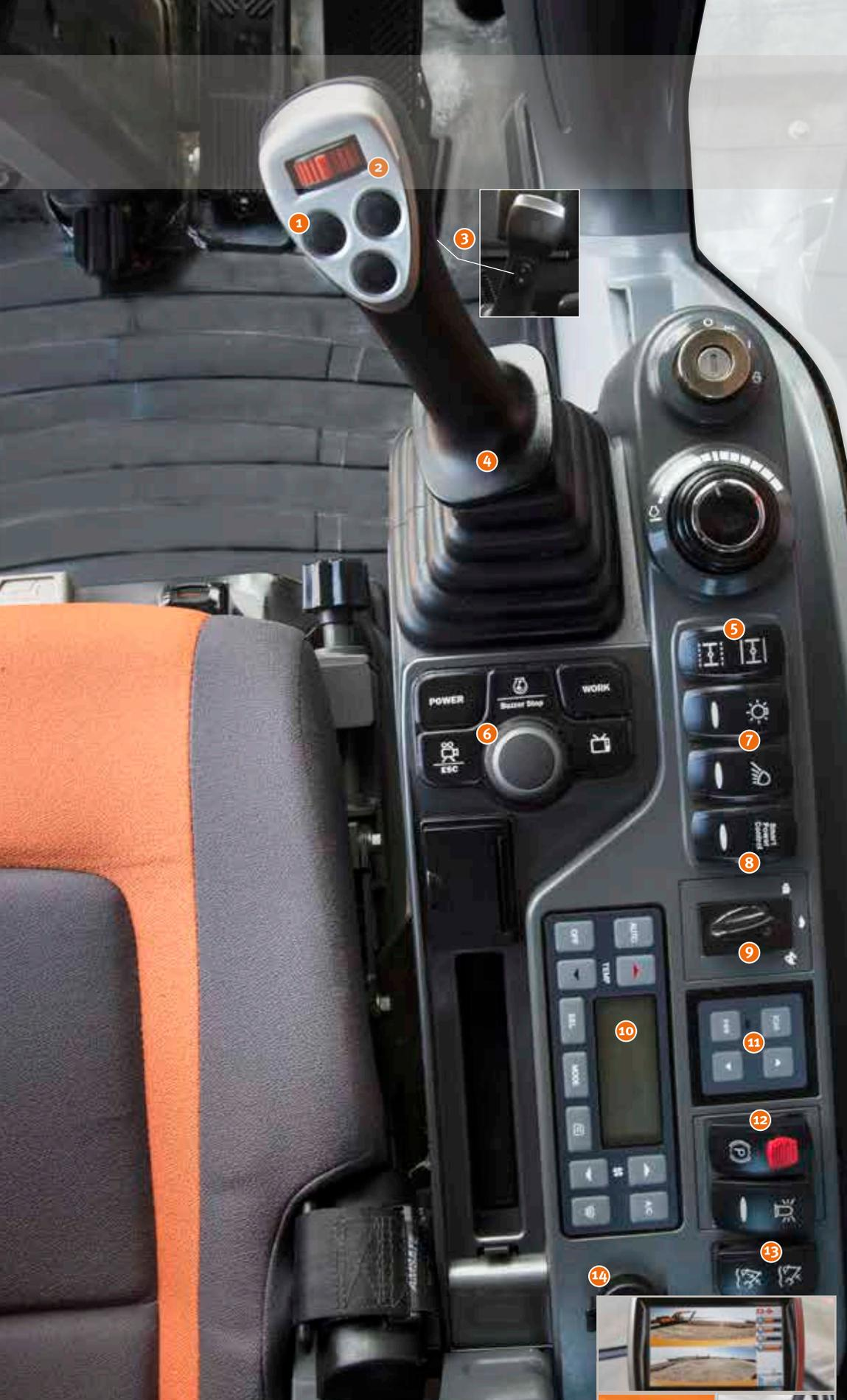
**Simple control:** Doosan's exclusive jog shuttle switch for easy and precise control over all machine functions.
