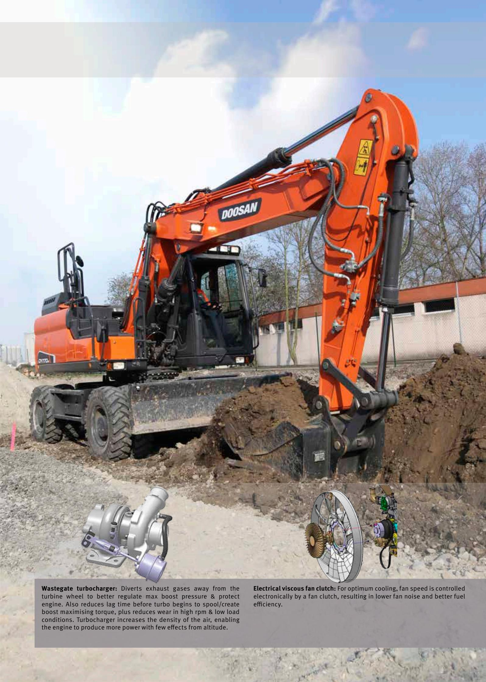
**Wastegate turbocharger:** Diverts exhaust gases away from the turbine wheel to better regulate max boost pressure & protect engine. Also reduces lag time before turbo begins to spool/create boost maximising torque, plus reduces wear in high rpm & low load conditions. Turbocharger increases the density of the air, enabling the engine to produce more power with few effects from altitude.
