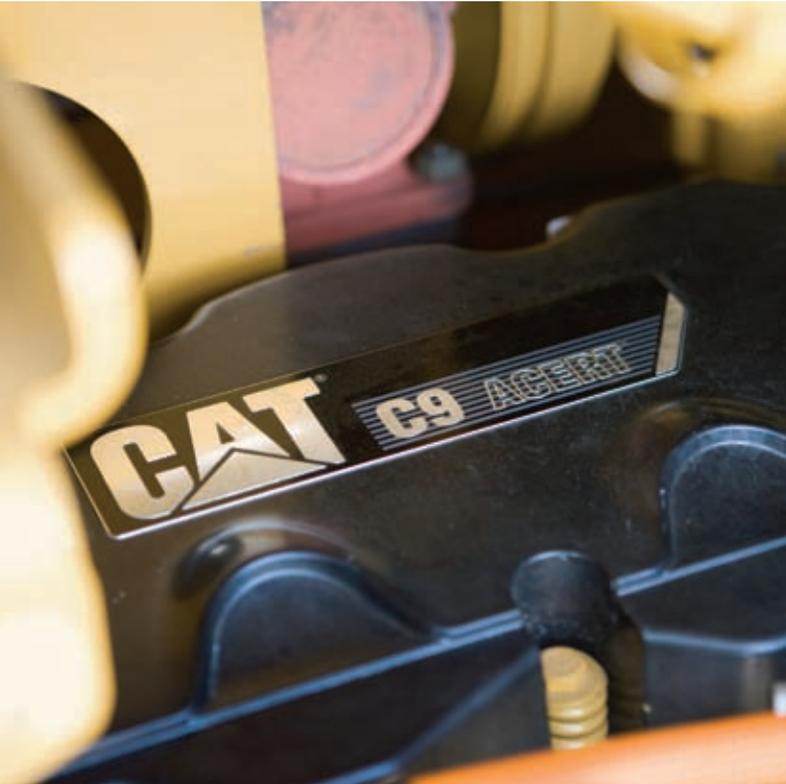
The D7E electric drive train is powered by a 235 hp Cat C9.3 engine with ACERT™ Technology. The engine utilizes a proven common rail fuel system for improved efficiency and fuel economy. Featuring the latest in Cat emissions reduction technologies, this engine meets U.S. EPA Tier 3, EU Stage IIIa and Japan MLIT Step 3 emissions regulations.
